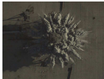
Figure 1. Formation of particle clusters in a jetting form during cylindrical dispersal of aluminum particles in air.
